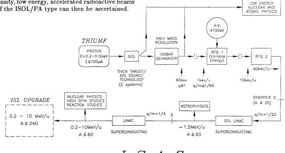
Fig. 2. Schematic representation of a revised ISAC Facility
