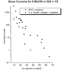
Figure 2: Intensities of ion beams with an energy of 5 MeV/amu out of the cyclotron for 2 different injectors versus atomic number (for the RFQ injector a total transmission from the source to the experiment of 10 % is assumed ).
