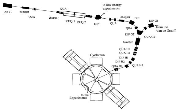
Figure 6: Beam line system from the end of the vertical part to the cyclotron.
