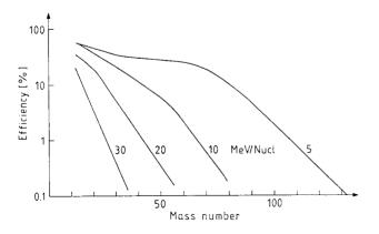
Figure 1: Stripper efficiencies for beams with different energies extracted out of the cyclotron versus ion mass.
