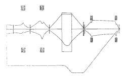
Figure 4: Beam envelope from the exit of the 200 kV acceleration tube to the entrance of the RFQ.
