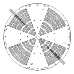
Figure 2. Trim coils of the VINCY Cyclotron.
