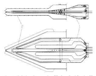
Figure 4. The horizontal cross section of the dee and anti-dee - 1 and 2, respectively, of the RF system of the VINCY Cyclotron defined by the median plane, and their vertical cross section defined by the symmetry plane of valleys V1 and V3.
