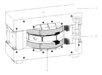
Figure 1. Magnetic structure of the VINCY Cyclotron: 1 - yoke, 2 elevation system, and 3 - main coil.
