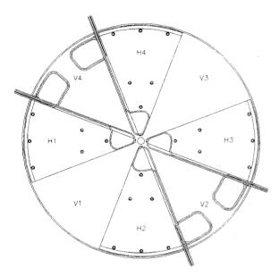
Figure 3. Harmonic coils of the VINCY Cyclotron.
