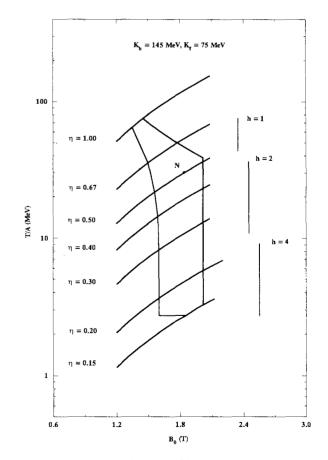
Figure 5. The operating range of the VINCY Cyclotron.
