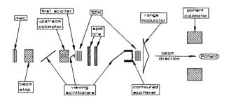
Figure 1: Diagram of the radiobiology and medical beam line (not to scale).
