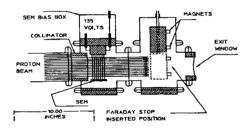
Figure 2 RERP Beamline Schematic (not to scale)
