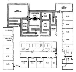
Fig 1. Layout of the Cyclotron facilities
