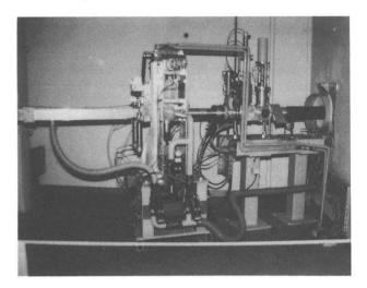
Fig 2. Solid Target Station installed in Solid Target Room
