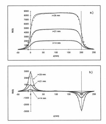
Figure 3: Axial distribution of the azimuthal (a) and axial (b) magnetic field components of the hexapole. Symbols - measured values, continuous lines - calculated curves.
