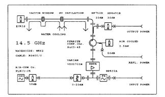
Figure 4: The microwave system of the ion source. OSC- oscillator, FM- frequency meter, KHPA - klystron high power amplifier.
