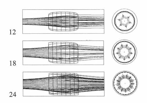
Fig. 5 Resonance zones and tubes of flux lines for different multipoles in two views. The multipole numbers are shown at left. The flux tubes start at the left side of the chambers.
