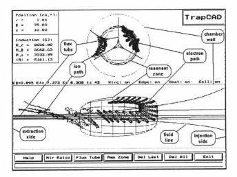
Figure 2: Example output of TrapCAD. 14 GHz, 1 T configuration.
