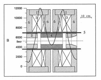
Figure 1: The layout of the magnetic system of the ECRIS and the calculated axial magnetic field (in gauss) along the source axis. 1,2,6 - iron components, 3 - coils, 4 - hexapole, 5 - insulator.
