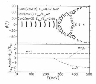
Figure 2: The bottom figure shows the effective energy gain per turn, normalized to the energy gain of the fundamental, for the fundamental, and additional  $2^{nd}$  and  $3^{rd}$  harmonic  $\lambda/4$  cavities as a function of energy. In the top figure particle trajectories in  $(E, \phi)$  space, plotted every one hundred turns, show how the initial phase band of  $\pm 10^{\circ}$  is split into three ~ 4° bands separated by 90°.
