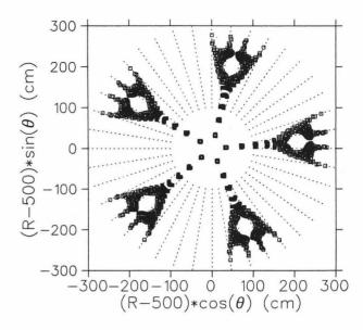
Figure 3: Shown are the five particle bunches per turn in TRI-UMF, starting from 500 cm (E = 140 MeV), and splitting into four bunches per spoke with the influence of the higher harmonic cavities; a  $2^{nd}$ ,  $3^{rd}$ , and  $8^{th}$ . Superimposed on the plot are the linac buckets, eight times the cyclotron frequency.
