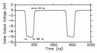
Figure 11: Measured output voltage from TRIUMF pulse generator.
