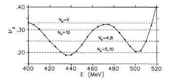
Figure 9: The vertical tune,  $\nu_z$ , as a function of energy for the TRI-UMF cyclotron. The dotted lines correspond to  $\nu_z$  values where the noted  $N_s$  values would produce resonant conditions.
