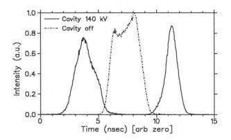
Figure 4: Experimental result showing the time spectrum of beam extracted from the TRIUMF cyclotron with (solid line) and without (dotted line) an additional  $4^{th}$  harmonic cavity  $(E_{G4}(R_f)/E_{G1}(R_f) = 0.88)$  phased to oppose the circulating beam.
