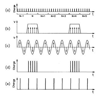
Figure 5: (a) Schematic showing the pulsed (b) and sinusoidal (c) fields required to create coherent growth at  $\nu_r = 1.25$  or  $\nu_z = 0.25$  for the h=5 bunch per turn time structure shown in (a). The extracted time structures for both the pulsed field (d) and the sinusoidal field (e) are also shown.
