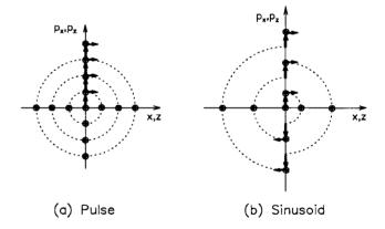
Figure 6: Schematic view of the motion in  $(x, p_x)$  or  $(z, p_z)$  at  $\nu_r = 1.25$  or  $\nu_z = 0.25$  for the deflecting fields shown in Fig. 5; in (a) from a pulsed field and (b) from a sinusoidal field. The vertical arrows show the particle deflections and the horizontal arrows indicate the direction of the  $2\pi/N_s$  phase advance.
