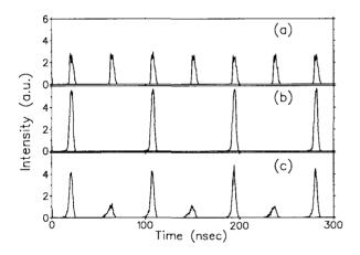
Figure 8: Experimental result showing the extracted time structure with and without the RFD  $(N_s=2)$ . In (a) with RFD off the bunches are separated by the normal period of 43 nsec. In (b) with RFD on the bunches are twice as bright and now separated by 86 nsec. In (c) the extraction foil is moved to extract a portion of beam from the neighbouring *satellite*.
