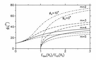
Figure 1: Final phase values for particles of initial phase  $\phi_o = 0^+, 10^\circ$  resulting from the addition of a higher harmonic cavity (m = 2, 3, 4, or 5) with peak energy gain  $E_{Gm}$  and phase opposing the fundamental. The  $\phi_o = 10^\circ$  results assume  $E_{G1}(R_o) = E_{G1}(R_f)$ .
