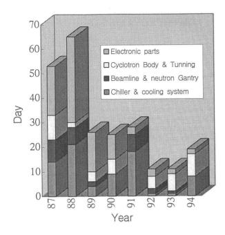
Figure 4: Failure days and parts
