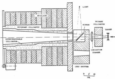
Fig.2 COLLIMATOR SYSTEM
