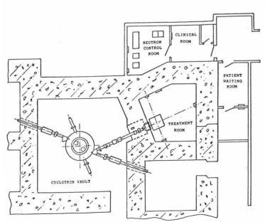
Fig.1 GENERAL LAYOUT OF NEUTRON
