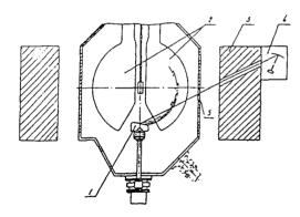
Figure 1 : Plane view of internal target position in IPPE cyclotron : 1 - target, 2 - dees, 3 - magnet yoke, 4 - infrared radiometer, 5 - window passing infrared radiation
