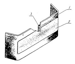
Figure 2: Isometrical view of internal target : 1 - cooper base of target, 2 - irradiated material, 3 - cooling ribs.
