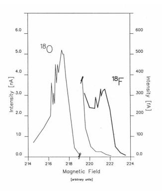
Figure 2 : Isobaric separation of <sup>18</sup>O and <sup>18</sup>F : intensity of the extracted beam versus the magnetic field of the cyclotron. Note that the intensity scale is different for <sup>18</sup>O (left scale, nA) and for <sup>18</sup>F (right scale, fA)
