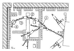
Figure 1: HRBL layout. 1-RIB production target; 2-degrader position; 3-main physics target; 4-QD spectrometer focal plane.
