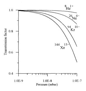
Figure 3: The transmission factor for some RIB.
