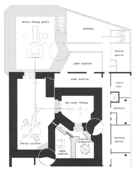
Figure 2: Proposal for a modernized neutron therapy facility
