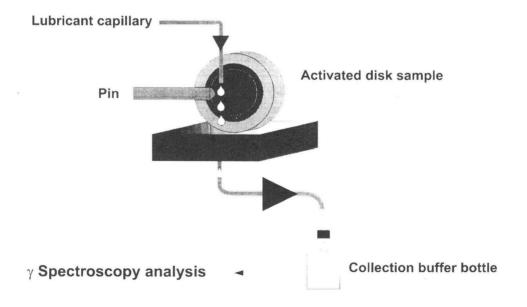
Fig. 3 : Schematic diagram of the test facility for lubricated pin on disk wear testing using TLA.
