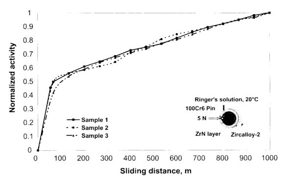
Fig. 4 : Normalised summed activity in collection buffer bottle versus sliding distance during wear testing of 3 different samples of nitrided Zircalloy-2.
