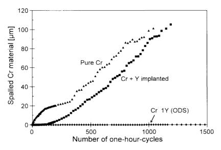
Fig. 1 Spallation behaviour measured using TLA of pure Cr, Cr implanted with 10<sup>17</sup> Y-ions/cm<sup>2</sup>, and Cr-1%Y<sub>2</sub>O<sub>3</sub> alloy upon thermal cycling at 1000°C [7].
