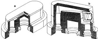
Figure 1: Sections through high power electroplated target (a) and low power target for irradiation of solids and stacks of foils (b).
