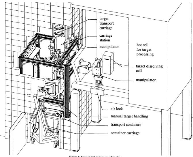
Figure 4: Service station for target handling
