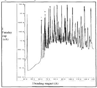
We can see on the same curve different charge states which have maximum value completely different.
