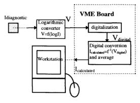
As seen before, the characteristic V=f(I) isn't linear on the whole scale. We have a non-linearity for low current (I< 10pA) and hight current (I>100 $\mu$ A). The theorical equation V=2\*log (I/Io) and the inverse equation (I<sub>calculated</sub>=Io\*10<sup>V4/2</sup>) can't be used.
