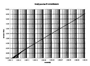
The different converters, for the same room temperature(25°C), have different characteristics for low current. Theses light differences are due to different values of Is.
