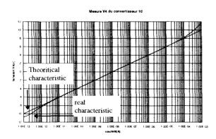
In practice, Ibias (amplifier bias current) and Is (reverse saturation current) make non-linearity in very low current (< 10pA). For the high current (I> $100\mu A$ ) the resistance Rs of diode causes a non-linearity.
