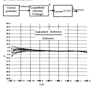
The precision for the low current (i<10<sup>-10</sup>A) decreases because diodes have different characteristics.
