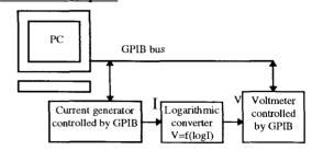
We acquire 1000 measurements of the characteristic V=f(I). We choose an average characteristic and a computer program calculates the characteristic I=f(V) with 4096 points. We use an analog to digital converter with 12 bits precision  $(2^{\Lambda^{12}}$ =4096 values). We put the values in an EPROM on the VME board.
