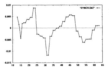
Figure 6. The relative deviations from linear increase,  $\Delta Br/(Br)$ , versus the magnet number of turn 2 to 5, showing two coherent synchrotron oscillations.
