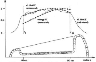
Figure 3. The radial characteristics of the electrical field E (measured and calculated) and voltage U of the cavities.
