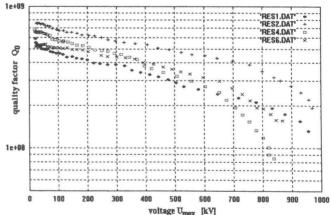
Figure 4. Typical curves of the unloaded quality factor of Tritron cavities versus the voltage amplitude at the last beam hole.
