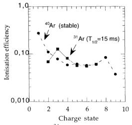
Figure 8: Comparison of  ${}^{31}$ Ar charge state distribution with the  ${}^{40}$ Ar distribution.
