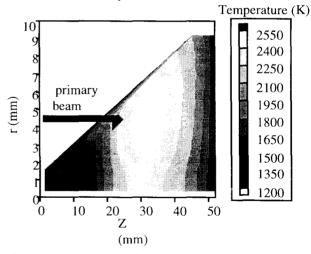
Figure 1: temperature distribution of a carbon target heated by a 2 kW Argon primary beam.
