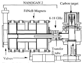
Figure 3: Schematic drawing of the first target ion source source system for the spiral project.
