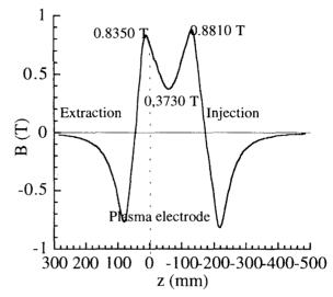
Figure 4: axial magnetic profile of the nanogan 2 ion source.
