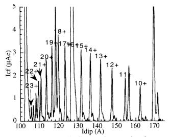
Figure 6: Charge state distribution of xenon when the source is optimised to produce  $Xe^{23+}$
