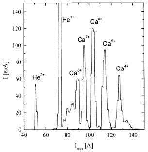
Fig.3 The spectrum of <sup>48</sup>Ca ions optimised for production of <sup>48</sup>Ca<sup>6+</sup>.
