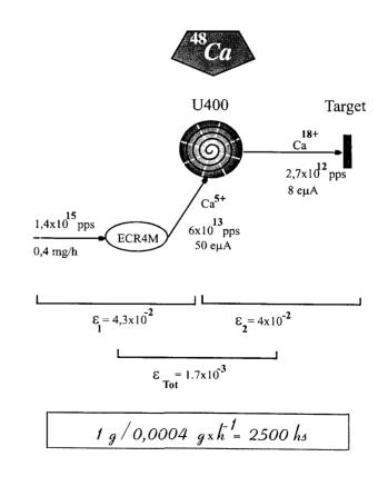
Fig.6. Efficiency of the ECR4M ion source and the U400 cyclotron with the  $^{48}$ Ca ion beam.
