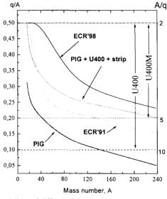
Fig.1 Potentialities of different high charge state and intensive ion sources for cyclotrons.
