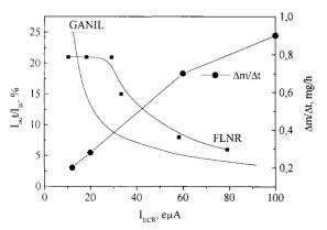
Fig.5 Experimental results for the bunching effect and consumption of metallic <sup>48</sup>Ca versus the ion beam intensity from the ion source.
