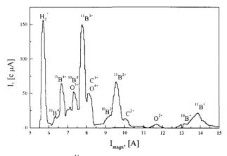
Fig.4 The spectrum of  ${}^{11}B$  ions produced from the  $C_2B_{10}H_{12}$  compound.
