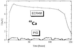
Fig.7 Intensity of the accelerated <sup>48</sup>Ca ion beams from the PIG [13] and ECR ion sources at a physical target.
