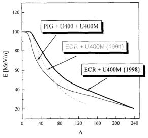
Fig.2 Dependence of the U400M ion energies on the ion mass.
