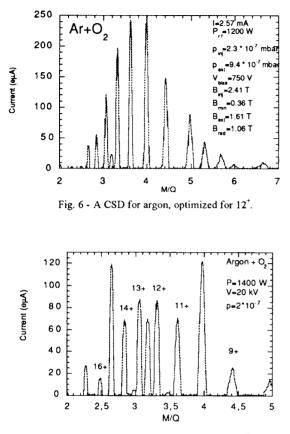
Fig. 7 - A CSD for argon, optimized for 16<sup>+</sup>.
