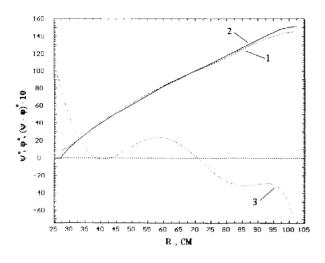
Figure 6:  $\psi$  (1) is phase of the main harmonic and  $\varphi$  (2) is a median line of iron sector along radius, $(\psi - \varphi)$  (3) is phase discrepancy along the radius.
