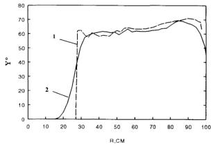
Figure 7: Spiral angle in dependence on cyclotron radius: 1 - geometry data of  $k_2=8$ model; 2 experimental values.
