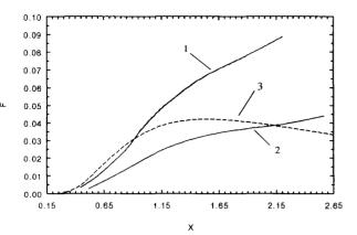
Figure 3: Flutter in dependence on nondimensional parameter  $x = r/Ng_h$ , where N = 4,  $1-2g_v = 386 \text{ mm}$ ,  $2g_h = 170 \text{ mm}$ ,  $h_1 = 108 \text{ mm}$ ;  $2-2g_v = 284 \text{ mm}$ ,  $2g_h = 145 \text{ mm}$ ,  $h_2 = 69 \text{ mm}$ ; 3-uniform magnetization for the case 1.
