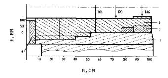
Figure 2: Shim profile in the hill and valley: 1-pole tip, 2-sector, 3-valley's shim, 4-central plug.
