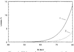
Figure 1: H<sup>-</sup> losses due to electromagnetic dissociation for two magnetic structures.
