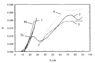
Figure 5: Flutter in dependence on cyclotron radius: 1 — the data of the measurements on model with straight sectors  $k_1 = 1.36$  (central part); 2 — the data of measurements on model with high spirallity  $k_2 = 8$ ; 3 — calculations on the base of proposed methodology with  $2g_v$ = 284 mm,  $h_1 = 69$  mm; 4 — calculations with  $2g_v = 386$  mm,  $h_1 = 108$  mm; 3a, 4a calculations with straight sectors.
