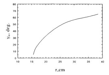
Figure 4: The ultimate spiral angle on dependence of radius for  $2g_v = 386mm$ ,  $2g_h = 170mm$ ,  $r = Ng_h x_{eff}$ , N = 4.
