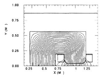
Figure 3 magnetic line distribution of CSR dipole
