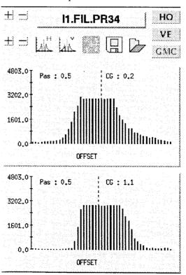
The horizontal and vertical profile monitor are displayed and their scale can be changed with the (+) or (-) push buttons. The shape can be frozen at any time, to be compared with the real time variations, and the HO or VE button displays the numeric values such as the center of gravity, the width ...
