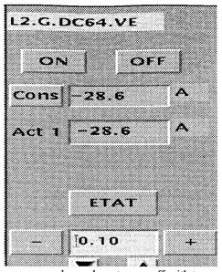
The power supply can be set on or off with two push buttons. The keyboard value is sent to the power supply, and the real read value is displayed into a text field just underneath. The push buttons (+) (-) can increase or decrease the current, and the increment value is managed by the two arrows.
