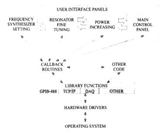
Figure 2: The RF Control System software architecture
