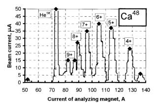
Fig.2. Spectrum of <sup>48</sup>Ca from ECR4M optimized for <sup>48</sup>Ca<sup>5+</sup>.
