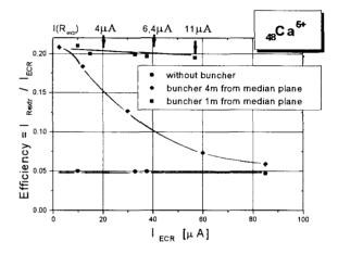
Fig.3. Efficiency of phase capture and acceleration in the cyclotron U-400 without buncher and with buncher installed in 1.1m and 4m from the median plane. ( $I_{R extr}$ - accelerated beam current at the final radius,  $I_{ECR}$ - injected beam current)
