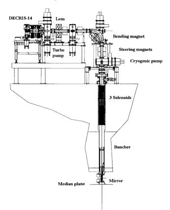
Fig. 4. The axial injection system of the U-400M cyclotron.
