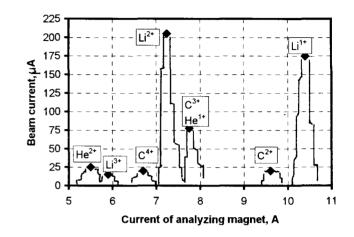
Figure 7. Li spectrum optimized on the maximum current of Li  $^{2+}$  beam required for acceleration.
