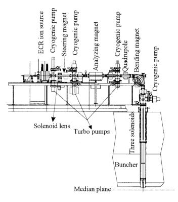
Fig. 1. The axial injection system of the U-400 cyclotron
