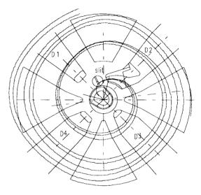
Fig.5. Diagram of the central region of the U-400M cyclotron and the trajectories of ions at dee voltage equal to 140, 150 and 170 kV.
