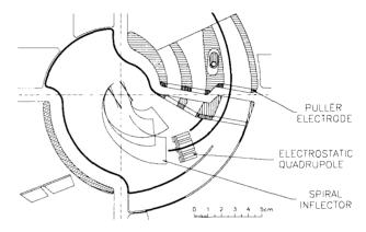
Figure 2: The position of the electrostatic quadrupole in relation to the spiral inflector and the puller electrode of SPC2.
