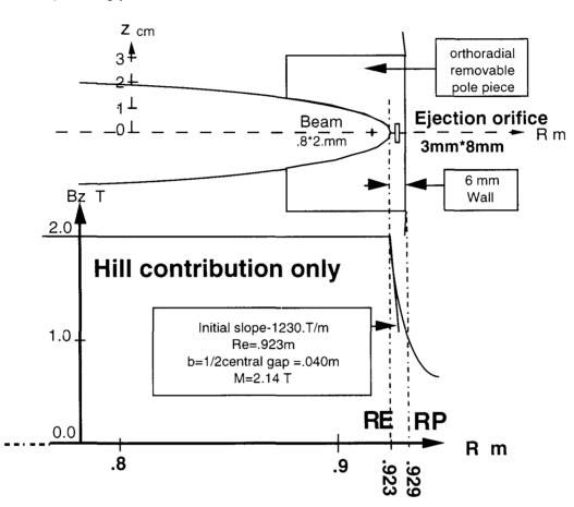
Fig 2: Vertical Hill cut aroud the pole radius showing the ideal beam which insures an ejection yield greater than 95% below the proper magnetic Hill contribution internal and external.
