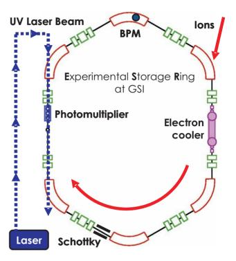
Figure 1: View of the ESR at GSI, Darmstadt. Laser beam and ion beam are brought in overlap in a straight section of the ring. The focus of the laser beam is adjusted to the position of the photomultiplier where the fluorescence signal of the ion beam is recorded. Also marked are the position of the electron cooler, the beam profile monitor (BPM) and the pickup electrode (Schottky). The ions revolve clockwise in the ring, the laser beam is counterpropagating to the ion beam.
