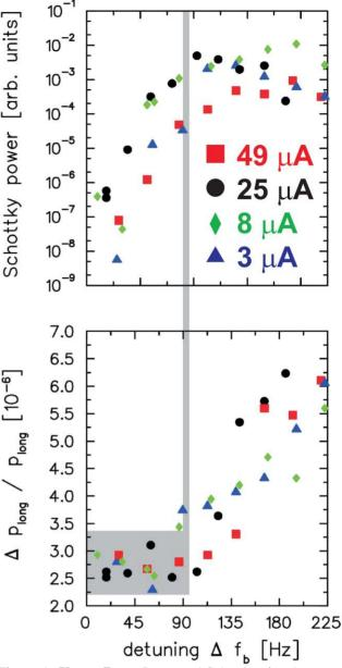
Figure 4: **Upper Part:** Integrated Schottky signal power versus detuning of the bunching frequency. The power of the Schottky signal is extracted from the Schottky spectrum, removing the constant background noise value and summing the signal for all peaks. For each detuning value a short time integration (usually 0.1 s) of the Schottky signal has been used to extract the corresponding power signal. The total signal power has been normalized to this integration time.
