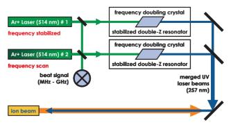
Figure 2: Laser system used for laser-cooling. The frequency of one laser beam is scanned relatively to the fixed frequency of another laser system. The scanning is controlled by measuring the beat signal of the two laser beams. Both laser beams are frequency-doubled separately using beta-barium borate crystals placed in a double-Z resonator geometry. After frequency-doubling, both beams are merged to one and brought in overlap with the ion beam.
