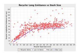
Figure 6: The calculated 95% longitudinal emittance (in units of eV-sec, assuming a Gaussian beam distribution) for the Recycler as a function of the beam intensity (units of  $10^{10}$ ). The pink and blue lines represent performance goals for cooling performance.
