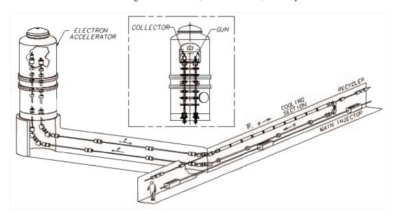
Figure 2: Electron Cooling insert in the Fermilab Recycler.
