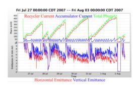
Figure 3: An operational week for the Recycler. In the top plot, blue is the Accumulator intensity, red is the Recycler intensity, and green is the sum (in units of  $10^{10}$ . In the bottom plot, red is the horizontal transverse emittance and blue is the vertical transverse emittance (both 95% normalized  $\pi$  mm mrad).
