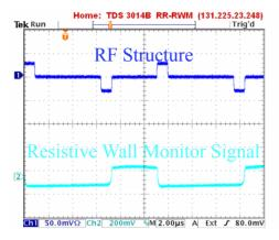
Figure 4: An oscilloscope view of the RF waveform (the integral creates a potential well) and the resistive wall monitor signal. The Recycler revolution period is  $11.13~\mu sec$ , so the  $20~\mu sec$  displayed shows more than 1 full turn.
