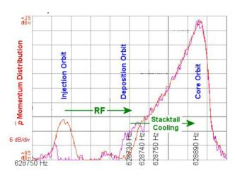
Figure 1: Stacktail Schottky profile vs. revolution frequency. Red trace with freshly injected antiprotons on the injection orbit, purple trace shows remnant antiprotons not picked up by the RF system and the resultant momentum displacement due to the Stacktail cooling.
