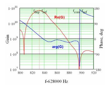
Figure 3: Gain profile of the Stacktail with real part of the gain function and phase as a function of revolution frequency.
