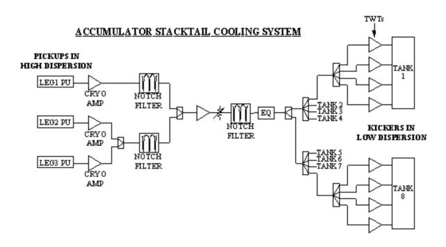
Figure 2: Block diagram of Stacktail cooling system.
