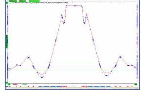
Figure 4: Dispersion corrections made to increase the slip factor. Red trace shows the new dispersion and blue data points correspond to the old lattice. Dispersion is changed in the negative wells and preserved at the flattop.
