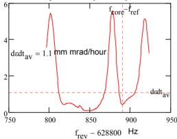
Figure 2: Emittance growth rate versus the particle frequency due to resonant heating at 3.3GHz. Vertical dash line shows the location of the core. Horizontal dash line shows average core heating rate due to this effect.
