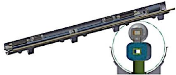
Figure 2: Schematic layout of placeholder cooling ring integrated above the collider ring in the same cryostat.
