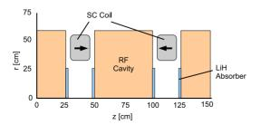
Figure 5: IDS-NF transverse cooling lattice cell, with alternating solenoids to create low- $\beta$  regions between RF cavities and thin, Be-coated LiH absorbers as cavity windows.
