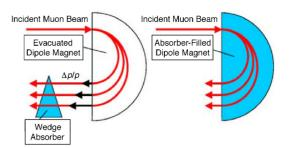
Figure 6: Two emittance exchange approaches: small beam with nonzero momentum spread is converted into more monoenergetic beam with transverse position spread. The reverse occurs in "Final Cooling." (Figure: Muons, Inc.)
