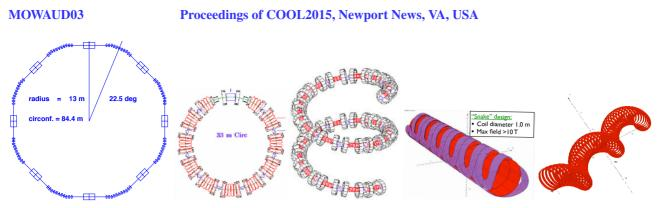
Figure 8: Examples of 6D cooling apparatus that have been shown to work in simulation: (left to right) quadrupole–dipole ring, "RFOFO" solenoid-focused ring, "RFOFO Guggenheim" helix, helical cooling channel (two versions).
