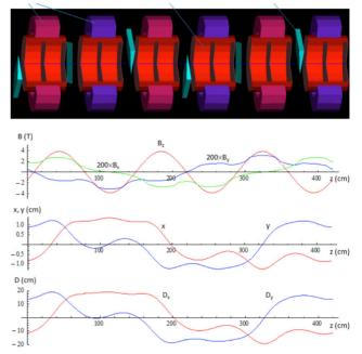
Figure 7: (top) HFOFO Snake lattice scheme, combining tilted solenoids with LiH-wedge and gaseous-hydrogen absorbers and RF cavities; (bottom)  $B_z$ , beam positions, and dispersion vs. distance along beam axis [38].
