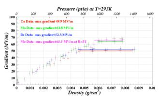
Figure 15: Observed dependence of maximum safe surface electric field in  $GH_2$ -pressurized 805 MHz cavity vs. hydrogen density and pressure for various electrode materials. Molybdenum electrodes were tested without (green points) and with (magenta) a 3 T axial field, with no observed degradation in maximum safe electric field [70].
