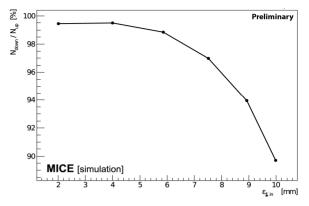
Fig 5: Muon beam transmission vs. input beam emittance for 200 MeV/c muon beam.
