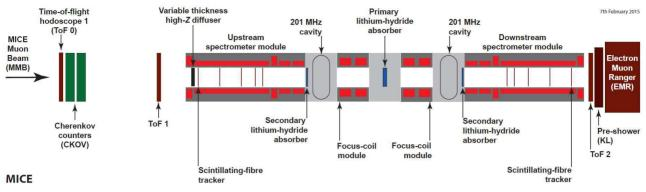
Fig 1: Schematic diagram of the final MICE cooling demonstration step.
