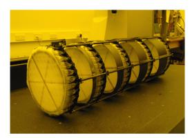
Figure 7: The MICE Tracker detectors showing the 5 stations each consisting of three planes of WLS fibres.
