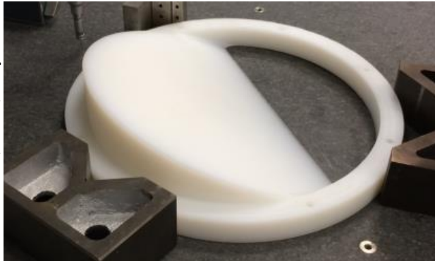
Figure 4: Polyethylene wedge piece machined for use in the MICE experiment. Wedge for mu2e would have similar dimensions. (Inner radius is \sim 20 cm).
