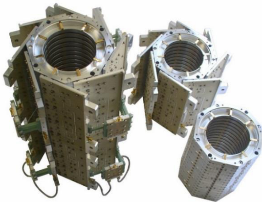
Figure 3: PU / KI of the high energy SC system for HESR. Right: One stack of 16 slot rings. Center: eight combiner boards are attached to the electrode lines. Left: Two stacks, boards are combined pairwise.
