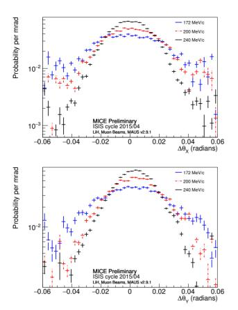
Figure 7: The results of the scattering analysis using data from all three nominal beam settings. Scattering widths are reported after application of deconvolution.
