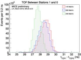
Figure 3: Top: The survival of muons after each stage of the selection. Bottom: The time of flight for muons between TOF0 and TOF1 for each of the nominal momentum points at which MICE will measure scattering at.
