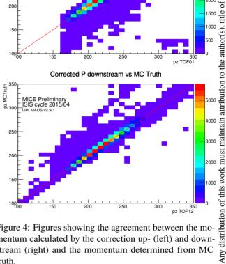
Figure 4: Figures showing the agreement between the momentum calculated by the correction up- (left) and downstream (right) and the momentum determined from MC truth.
