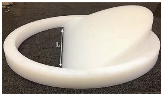
Figure 6: Photo of 1/2 of polyethylene-wedge absorber.
