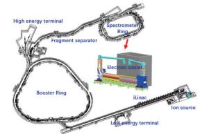
Figure 1: Layout of the HIAF accelerator and its cooler.
