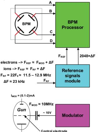
Figure 1: The structure of the BPM system.
