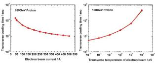
Figure 2: The transverse cooling time as a function of the electron beam current (left) and the transverse temperature of electron beam (right).
