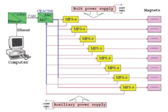
Figure 1: Structure of power module MPS-6.
