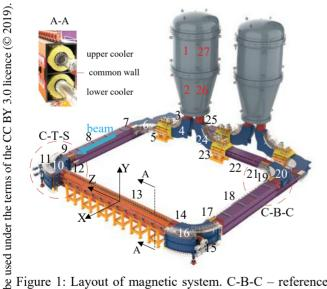
Figure 1: Layout of magnetic system. C-B-C - reference may segment, C-T-S – multifunctional segment.
