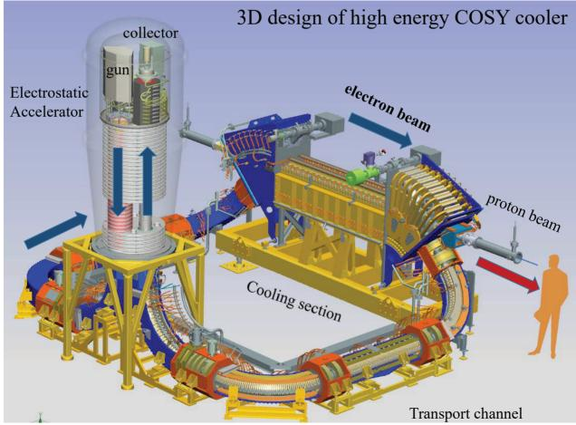
Figure 1: 3D design of 2 MeV COSY cooler.
