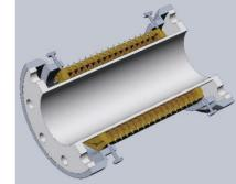
Figure 2: Schematics of pickup (kicker) with internal sealing using ceramic vacuum chamber.
