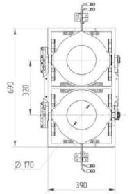
Figure 2: Cooling solenoid cross-section.
