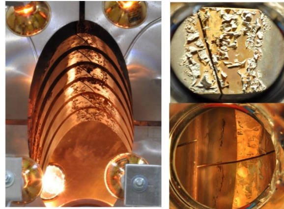
Figure 4: Left: Collimator front view with Ni-aperture. Right: Photo from the exit, vertical position, and entry at horizontal position (picture on the bottom).
