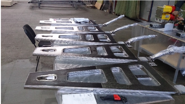
Figure 6: The blocks of azimuthal trimming coils.
