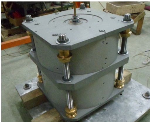
Figure 7: The DECRIS-PM magnetic system.
