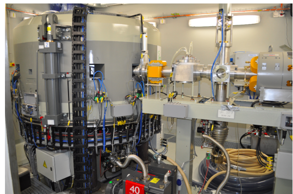
Figure 1: The compact medical PET cyclotron and its research beam line installed at the Bern University Hospital.
