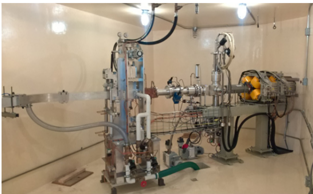
Figure 6: Cyclone® 70P: cyclotron beam transport line and the solid target station
