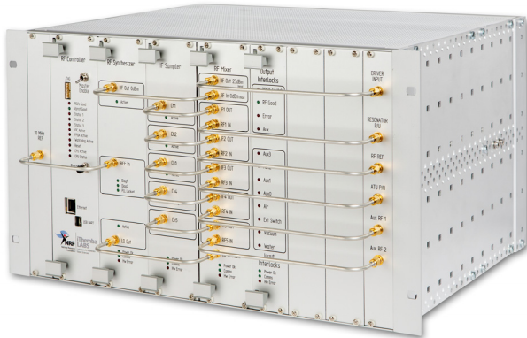
Figure 1: A photograph of the new digital low-level RF control system.
