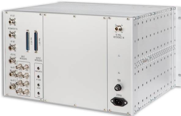
Figure 2: A photograph of the rear side of the new digital low-level RF control system.
