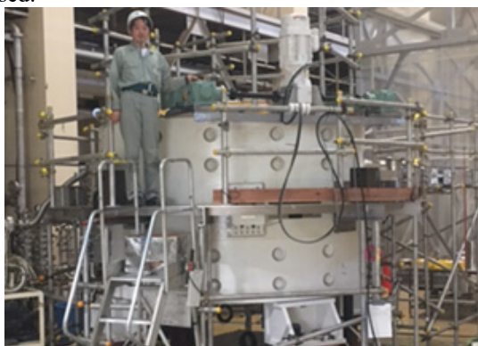
Figure 1: Superconducting cyclotron magnet. Diameter of the yoke is 2.8 m.
