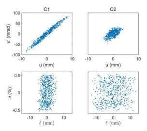
Figure 7: Vertical (top) and longitudinal (bottom) emittance plots at the first acceleration gap.
