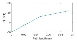
Figure 6: Design of the C2 inflector, showing how the tilting parameter Q changes along the path length.
