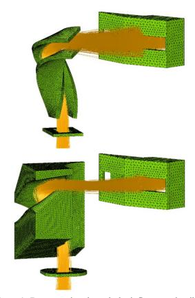
Figure 1: Beam passing through the inflector and striking the vertical slit in an ordinary spiral inflector (top), and in a field gradient inflector with vertical focusing (bottom).
