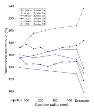
Figure 8: Experimental transmission through SPC2 when using the field gradient inflector C2, compared to the transmission with the ordinary spiral inflector C1.
