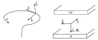
Figure 2: Standard inflector coordinate system (left) and the positioning of the electrodes to create the central field  $E_0$  (right).
