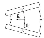
Figure 3: Electrode cross sections in the transverse plane. Traditional parallel electrodes (left) keep the electric field as uniform as possible, while tilting the electrodes (right) intentionally creates electric field gradients.
