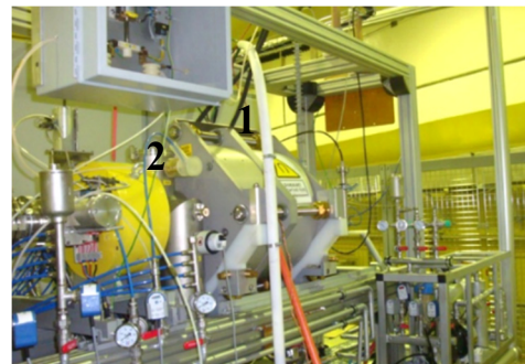
Figure 4: DECRIS-PM source at HV platform, where 1- the source body, 2 – focusing solenoid.
