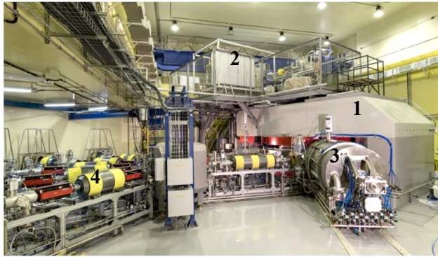
Figure 2: DC280 cyclotron, where: 1- main magnet, 2-HV injection system, 3-RF resonator, 4- beam lines.
