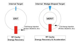
Figure 1: Schematic diagram of ERIT and MERIT scheme
