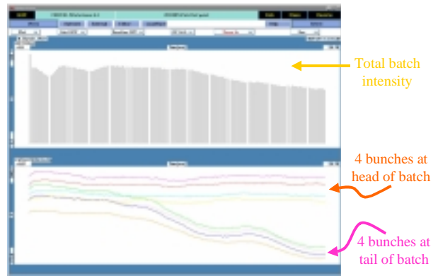
Figure 7: IBMS acquisition for a complete SPS cycle, showing beam loss at the tail of the batch.
